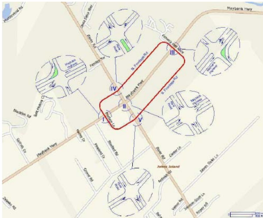
Schematic Plot of Revised Lane Configurations – Alternative C (Image produced by The LPA Group Incorporated)
